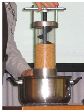
Olds Elevator (full-bore flow)
